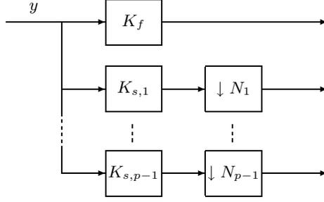
Figure 7: AFB  $E_k(K)$  with decomposed controllers
