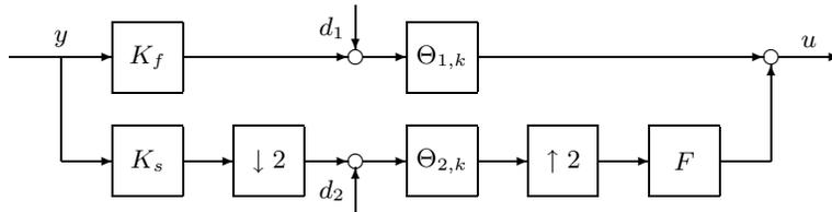
Figure 3: Decomposed controller in a subband coder form
