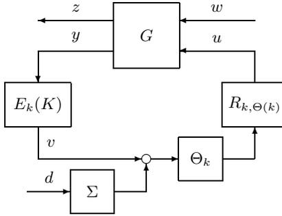
Figure 5: Networked control system with quantization noise
