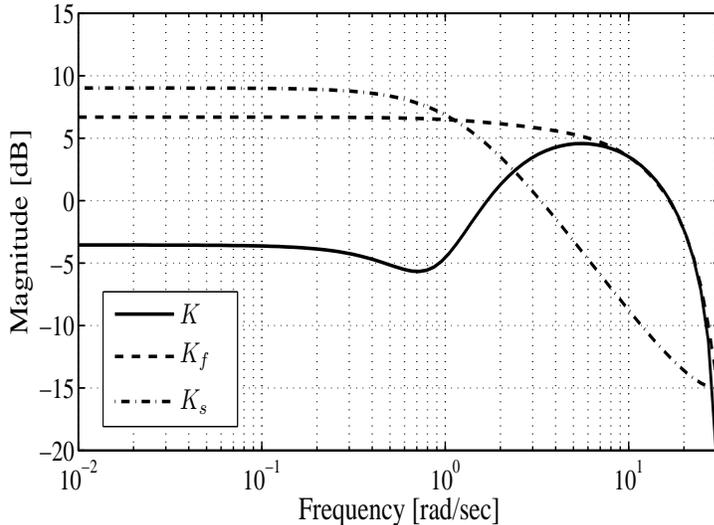
Figure 9: Frequency responses of the original controller  $K$ , the fast controller  $K_f$ , and the slow controller  $K_s$
