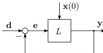
Figure 1: Discrete-time feedback control system.
