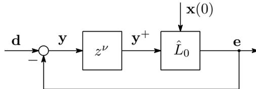
Figure 3: Equivalent system with the inverse system  $\hat{L}_0$  of  $L_0$ .
