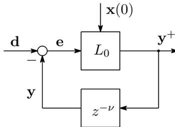
Figure 2: Equivalent system with the biproper system  $L_0$ .
