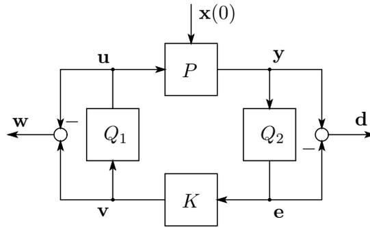
Figure 6: Model of a networked control system including quantizers.
