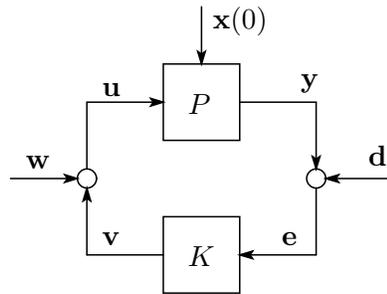
Figure 2: Model of a networked control system.
