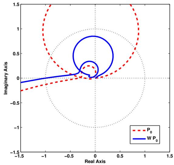
Figure 14: Nyquist plots of the torsion disk and the weighted plant.
