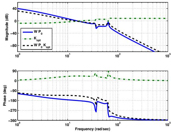
Figure 15: Bode plots of the weighted plant + controller.
