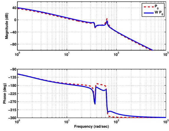
Figure 13: Bode plots of the torsion disk and the weighted plant.
