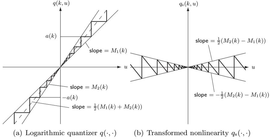
Figure 2: Decomposition of a quantization function for  $m = 1$
