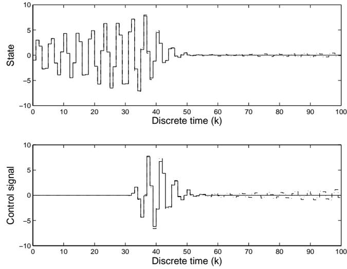
Figure 6: State trajectory and control signal versus time for the case of  $\bar{u} = 0$  (solid line) and  $\bar{u} = 1$  (dash-dot line)
