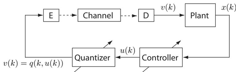
Figure 1: Adaptive control scheme with a time-varying quantizer, where E and D represent the encoder and the decoder, respectively.
