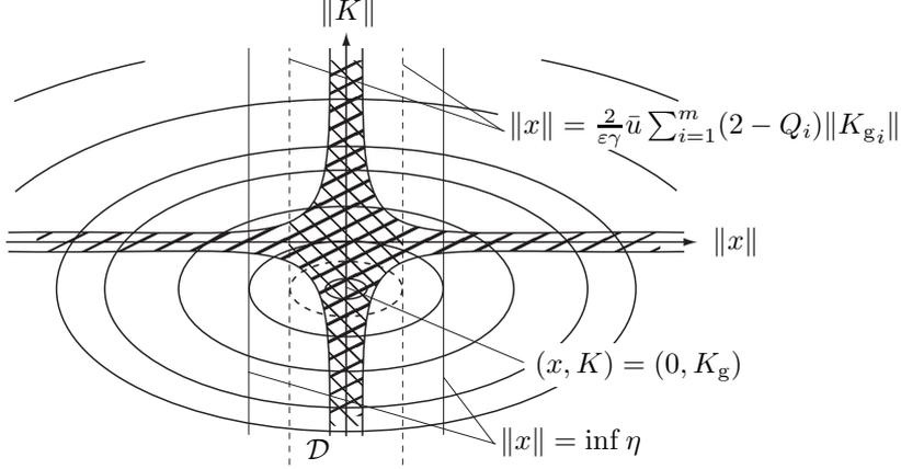
Figure 4: Visualization of the Lyapunov level sets. The shaded area indicates the region in which the quantizer produces null control effort ( $K(\cdot)x(\cdot) \leq \bar{u}$ ).
