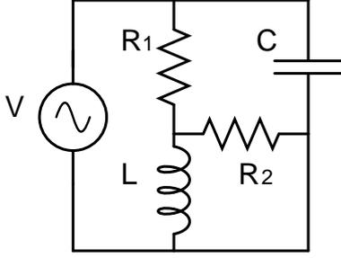
Figure 3: An RLC circuit that has hybrid equations with index one (Example 4.10).
