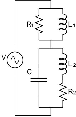
Figure 5: An RLC circuit that has hybrid equations with index zero (Example 4.11).
