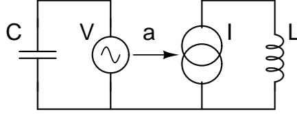
Figure 8: A linear circuit that has hybrid equations with index two.
