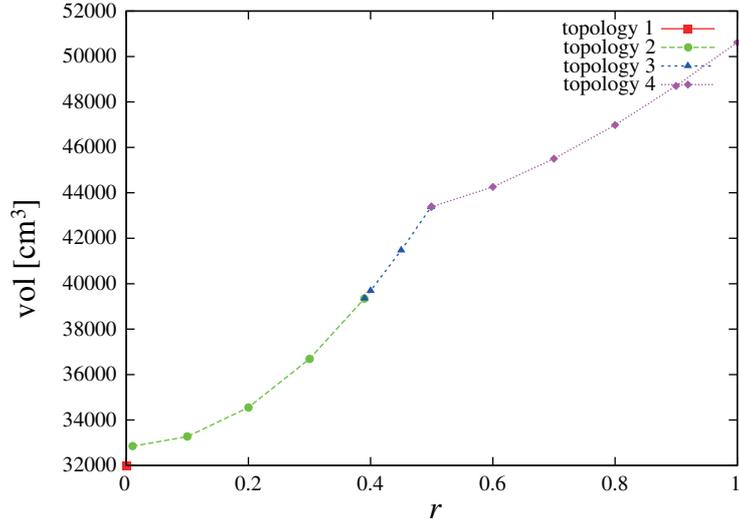
(a) Variation of the optimal structural volume with respect to the level of uncertainty.
