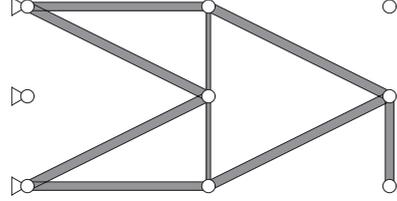
Figure 2: The optimal solution of the 22-member truss without considering load uncertainties.
