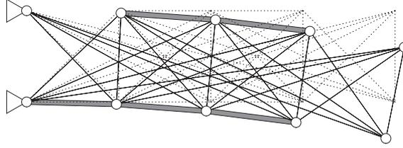
Figure 5: Worst scenario for  $\alpha = 3$  when the two missing members in Figure 3(b) are specified to be absent ( $\rho = 0$ ). The limit load factor of this scenario is 6.2500 ( $> \lambda_{\min}(3, \tilde{\mathbf{x}})$ ).
