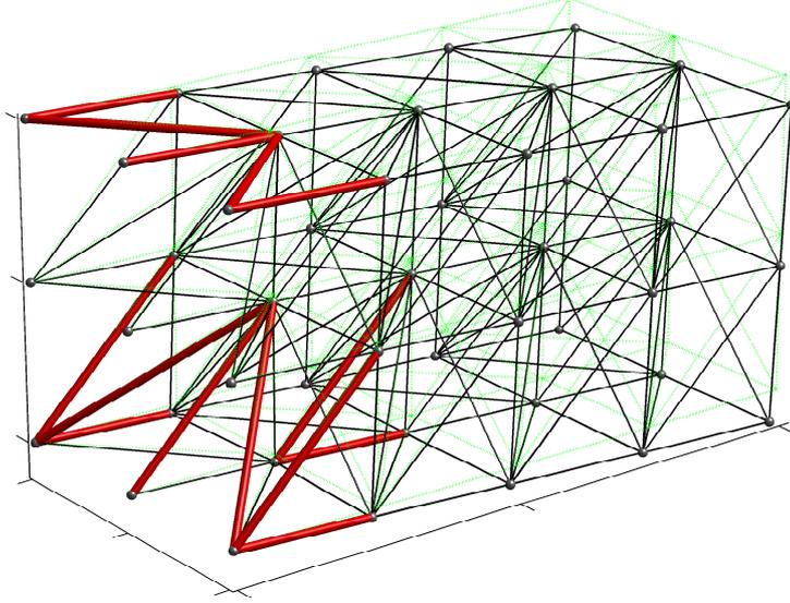
Figure 8: The collapse mode of the nominal structure of the space truss example. The members represented by thick lines experience plastic deformations.
