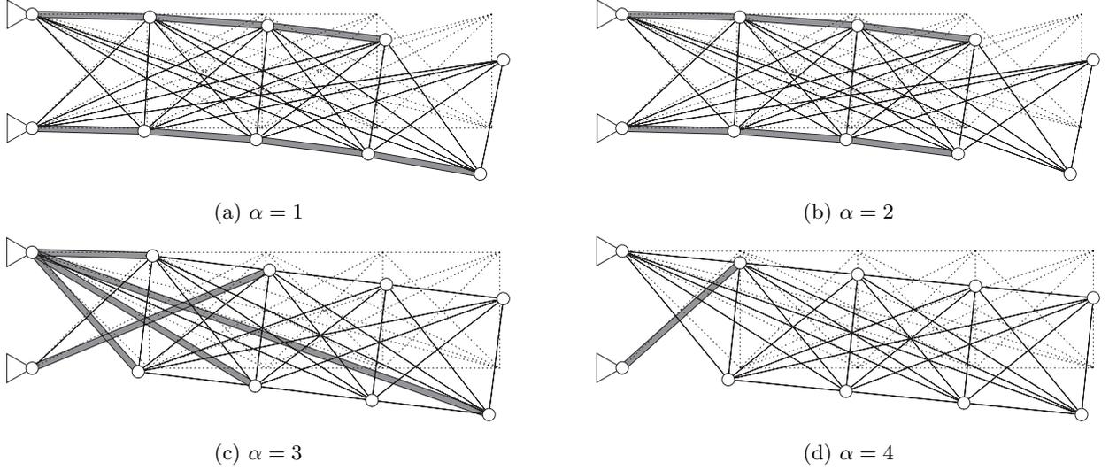
Figure 3: Worst scenarios and collapse modes of the plane truss example ( $\rho = 0$ ).
