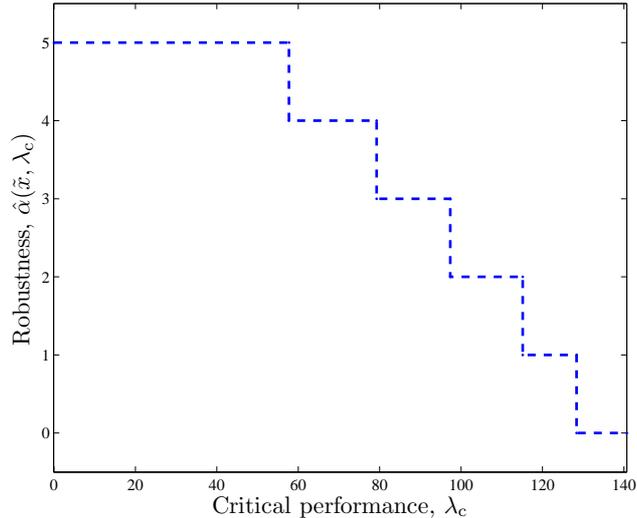
Figure 10: Trade-off relation between robustness and the critical performance for the space truss example.
