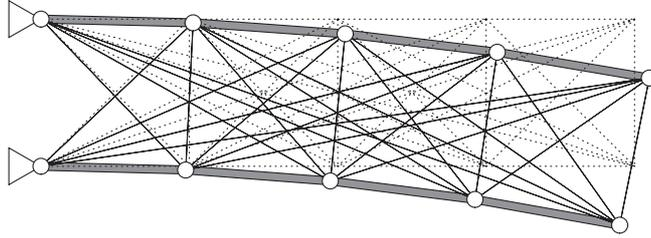
Figure 2: The collapse mode of the nominal structure of the plane truss example. The members represented by thick lines experience plastic deformations.
