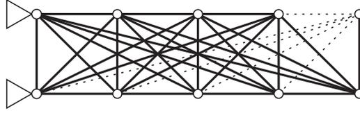
Figure 4: Worst scenario of the plane truss example for  $\alpha = 5$  ( $\rho = 0$ ).
