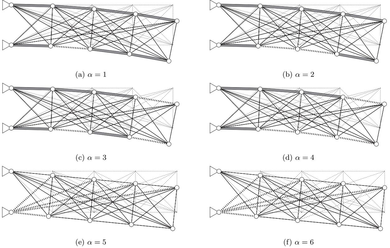
Figure 6: Worst scenarios and collapse modes of the plane truss example ( $\rho = 0.2$ ).
